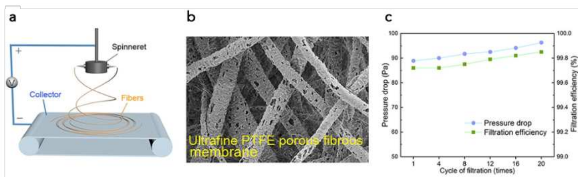
Figure 2.12 Schematic representation of ECS fabrication process (a); SEM micrograph of porous fibers (b); membranes filtration performance (c). Reprinted (adapted) from [89], Copyright (2021), with permission from Elsevier.
