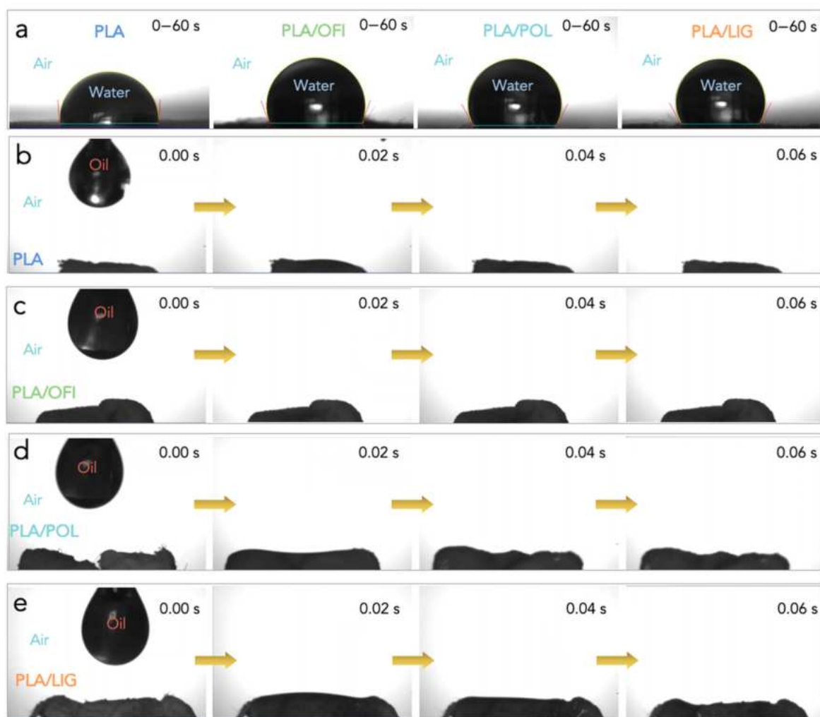
Figure 4.2.2.5 3D fibrous structures water and oil wetting behaviour: water wettability in air (a); wettability of oil in air of PLA (b), PLA/OFI (c), PLA/POL (d), PLA/LIG (e).
