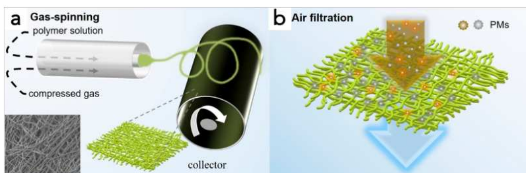
Figure 2.13 Schematic representation of SBS technology (a) for the production of nanofibers membranes for air filtration application (b). Reprinted (adapted) with permission from [53], Copyright (2020), American Chemical Society.
