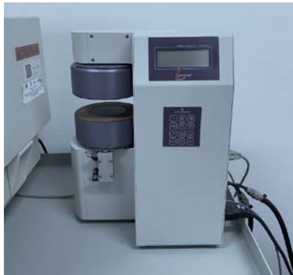
Fig. 4.8 Fox 50 Heat Flow Meter - TA Instrument.
