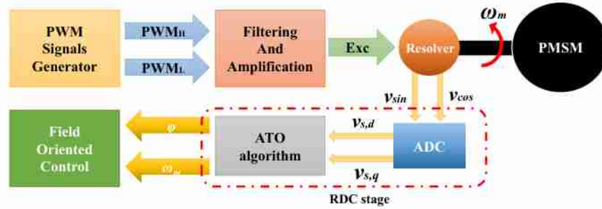
Fig. II. 10: Resolver excitation system and Resolver-to-digital conversion stage.
