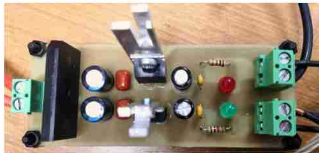
Fig. II. 17: External \pm 15 V power supply board realized at the Rapid Prototyping Laboratory, at the university of Palermo, Palermo, Italy.
