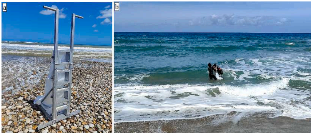
Fig. 3. (a) Streamer trap used to measure field LST rate. (b) Example of acquisition survey at the Cefalù Site performed on 2 nd April 2024 with a significant offshore wave height of 0.6 m, direction 297°N and period of 8 s.
