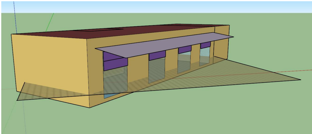
Fig. 84. Energy Plus Model with Shadings Covering the 40% of the Windows
