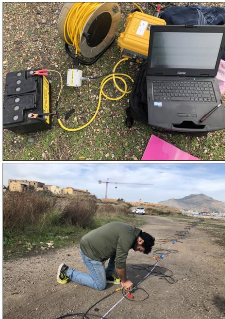
Figure 44: Active seismic data acquisition phase: at the top, the instrumentation used, at the bottom, the preparation phases of an array.
