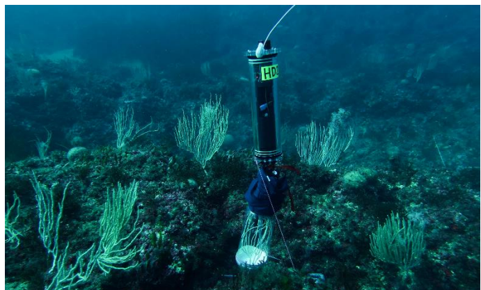
Figure 1. Benthic chamber and environmental data logger station measuring on a colony of Eunicella singularis in the MPA of Capo Gallo - Isola delle Femmine.
