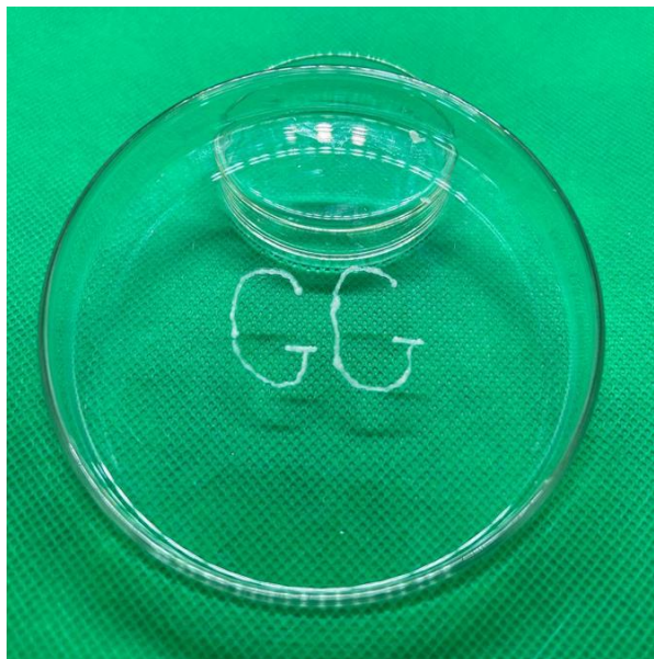
Figure 68. Macroscopic demonstration on H_{nc}E injectability, by writing with this hydrogel.
