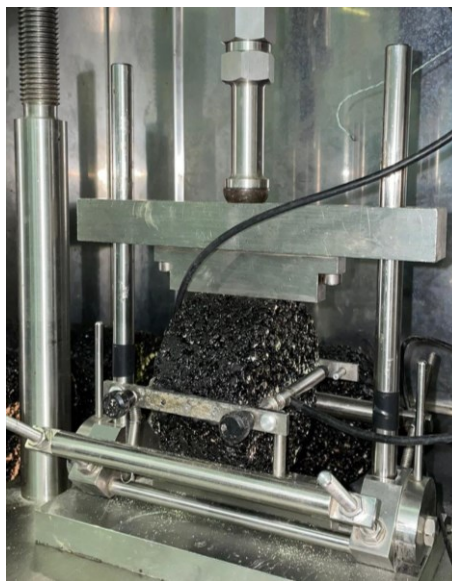
Figure 3. 5 ITFT test setup.
