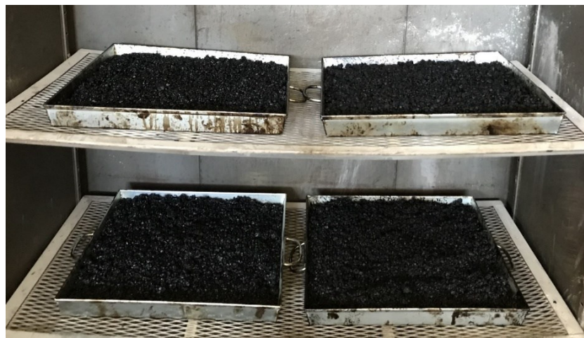
Figure 4. 3 Loose asphalt mixture ageing.
