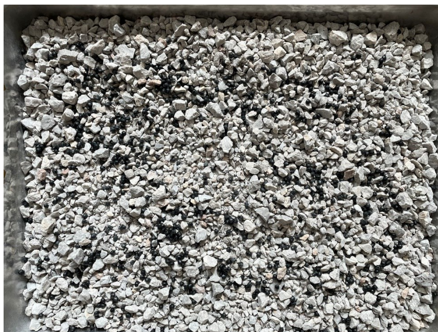
Figure 5. 9 GRP granules placed over the hot aggregates.
