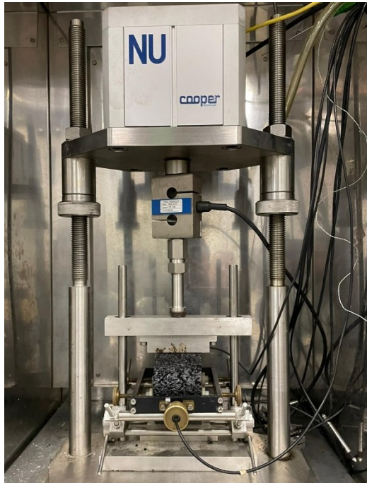
Figure 3. 3 ITSM test setup.
