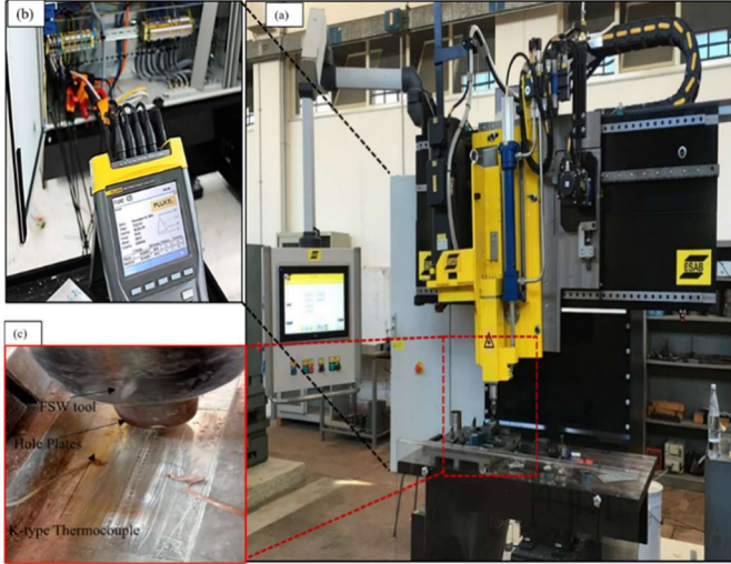
Fig. 1. (a) ESAB Legio 3 ST machine for FSW (b) The machine's enclosure and Multimeter for the measurements exhibited both current clamps and tension alligator clips. (c) Fixture layout for the FSW process and K-type thermocouple.
