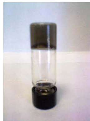
Fig. 1 Hydrogel of SWNTs prepared with p -dodecyloxy-benzylidimethylamine oxide (pDoAO).
