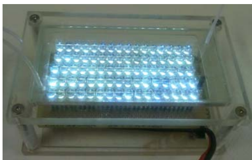
Figure 1 - Photochemical microreactor with white LED illumination
