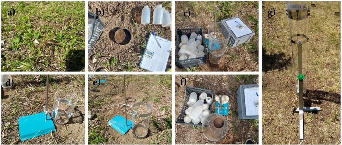
722 Fig. 1. View of the experimental site at the time of the experiment (a) and of the infiltration 723 runs with a height of water pouring of 0.03 m (b), 0.25 m (c), 0.5 m (d), 1 m (e), 1.5 m (f) and 724 2 m (g)
