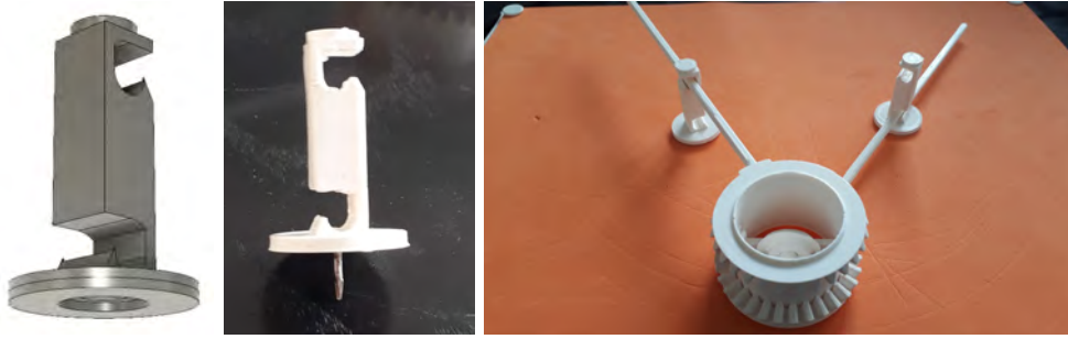
Figure 11. Left: model of a peg for a finite focus. Center: a 3D printed peg, including inside a drawing pin (glued in the bottom hollow). Right: bisector mechanism with two pegs constraining the passage of the rods.
