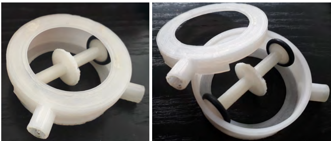
Figure 10. A bisector machine using rubber wheels to avoid gears. The two rubber wheels share the same axis but can rotate independently.
