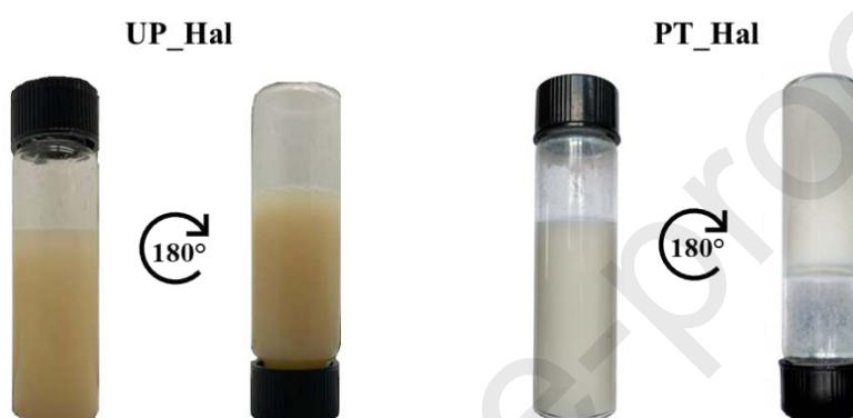
Fig. 3. Inversion test of PT_Hal and UP_Hal 1 wt%.
