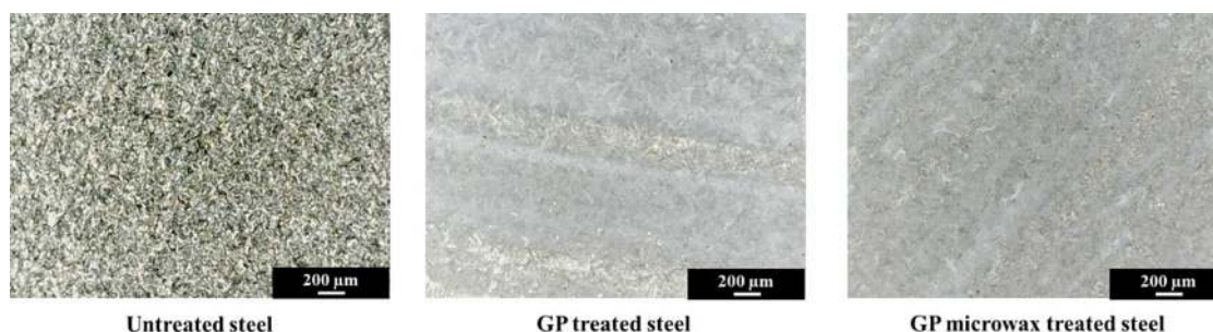
Fig. 1. Optical micrographs of untreated steel and sheets coated with HNTs based geopolymer and beeswax/HNTs microparticles based geopolymer.
