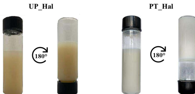
Figure 4.3. Inversion test of PT_Hal and UP_Hal 1 wt%.
