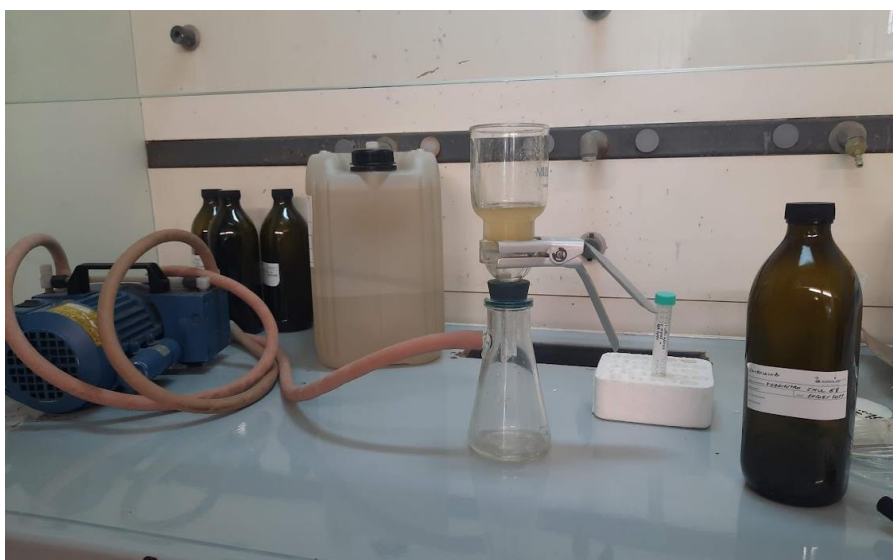
Figure 2.1. Groundwater filtration through a filtering complex connected to a vacuum pump
