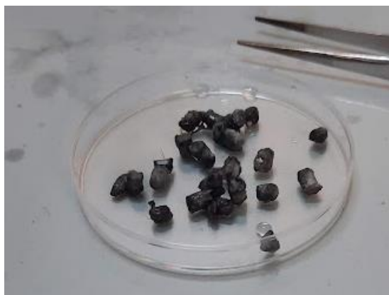
Figure 5.10. PLA ES scaffolds retrieved after 60 days of incubation at 20 m depth in the aquifer, site S2.
