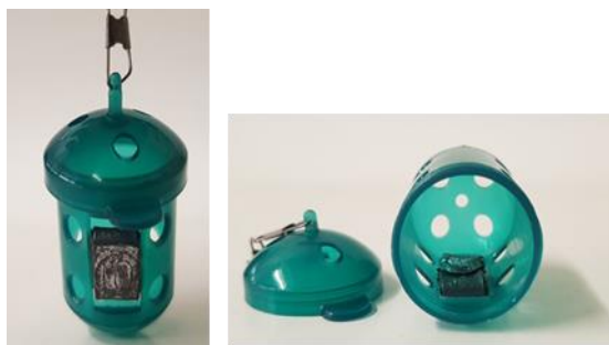
Figure 5.4. Plastic containers used to sink the scaffolds in groundwater
