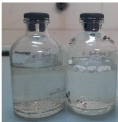
Figure 5.3. Microcosm containing groundwater and PLA ES scaffolds (right) and control microcosm with groundwater only.
