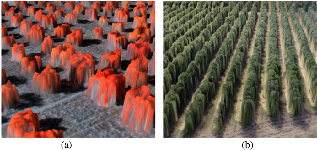
Figure 3. 3D representation of a traditional plantation generated with a multispectral sensor (a) and a row plantation generated with a visible light camera (b). Data from (Torres-Sánchez et al., 2015a).
