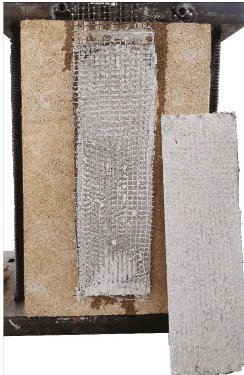
Figure 3.50: Observed failure mode C for specimens of group BL_DSB2.
