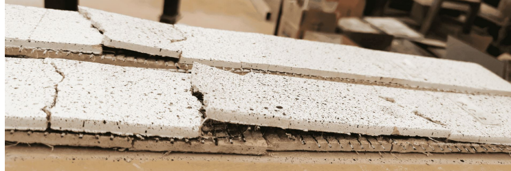
Figure 3.17: Delamination at the fibre-mortar interface for coupons of group BL_TH.
