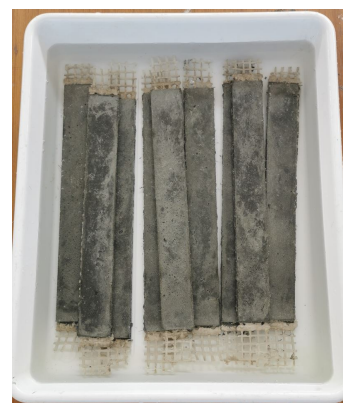
(d) curing in water for GFRCM with cement based mortar
