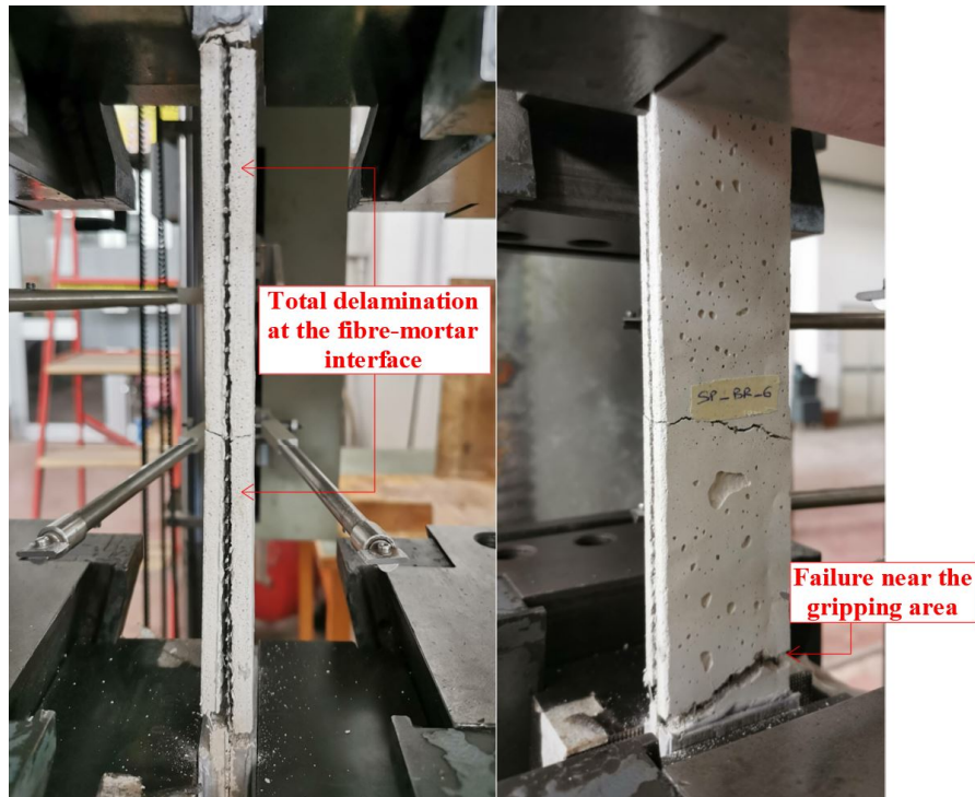
Figure 3.9: Failure mode of specimens BL_TF_6.
