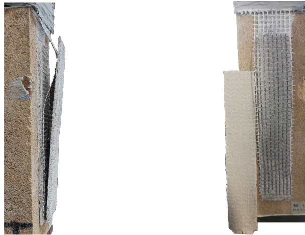
(a) debonding at fibre-matrix interface (b) detachment of the mortar layer
