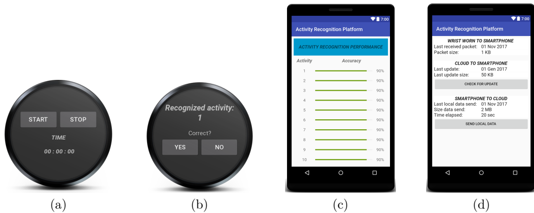
Figure 4.1: Smartwatch and smartphone Android applications. (a) The overall activity recognition process starts by pressing the start button on the wrist-worn interface. (b) Data are processed by the smartphone and the user is asked about the correctness of the classification. Detailed information about the recognition results (c), and data transmission statistics (d) can be examined through the smartphone-side app.
