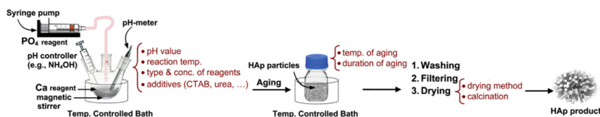
Figure 4.16 Steps of hydroxyapatite preparation via wet chemical method, from Sadat-Shojai et al. 2013
