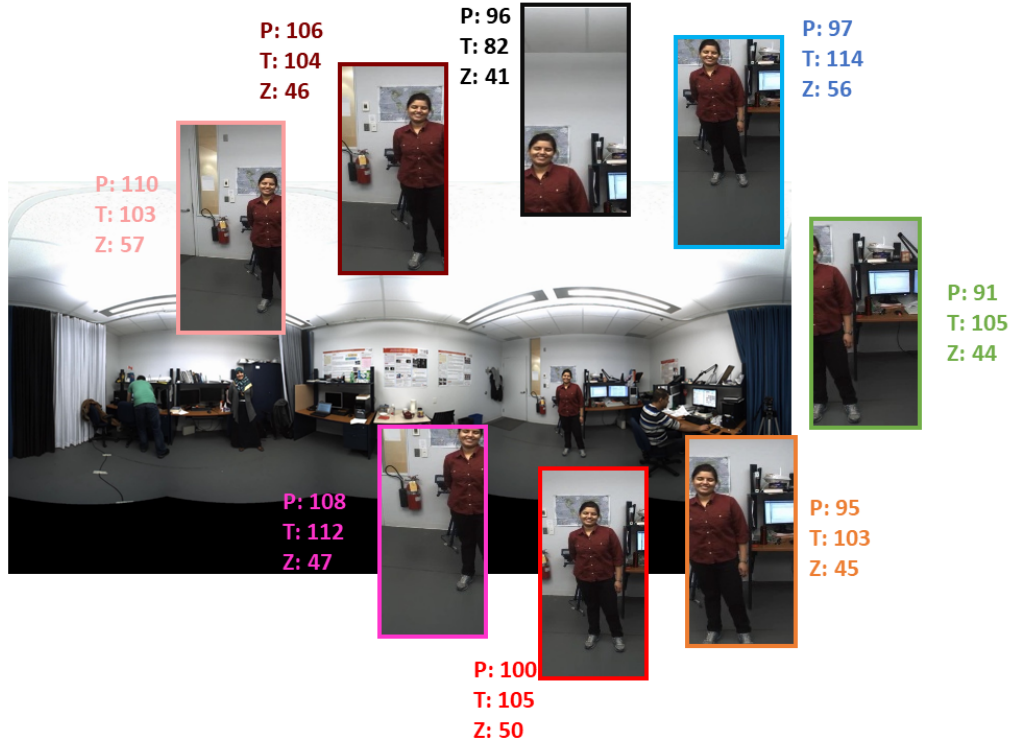
Figure 3.8: The image shows an equirectangular image and a set of views acquired by different vPTZ cameras with the reported parameters.
