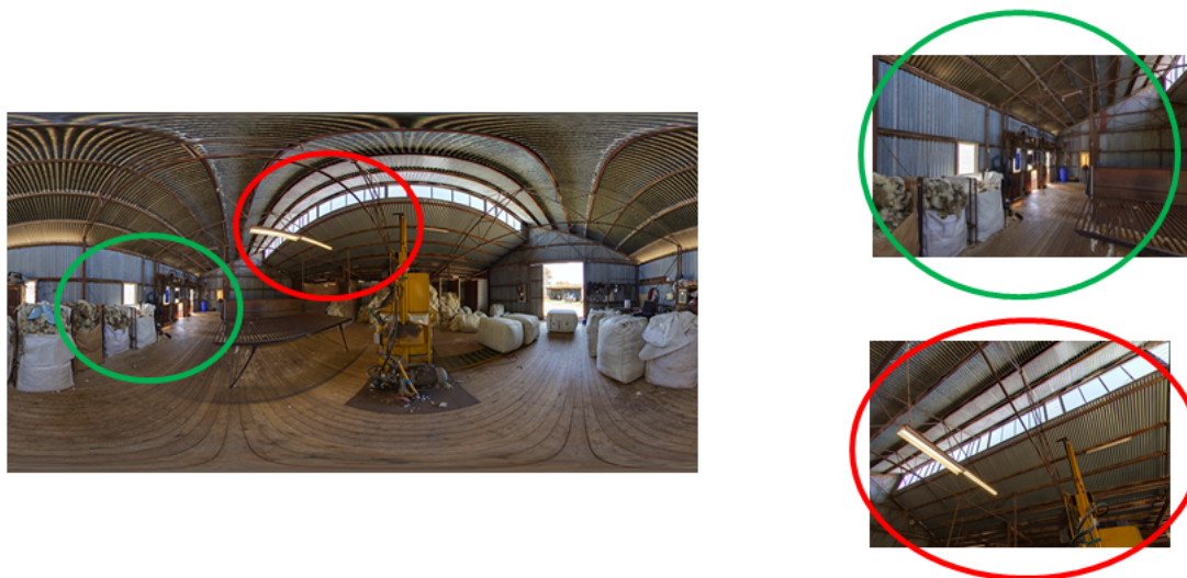
Figure 3.3: The gnomonic projection allows the mapping of a specific portion of the spherical view onto a tangent plane. By varying the tangent plane, it is possible to get different projections of the spherical surface. The red and the green circle show the projected portions of the equirectangular image.
