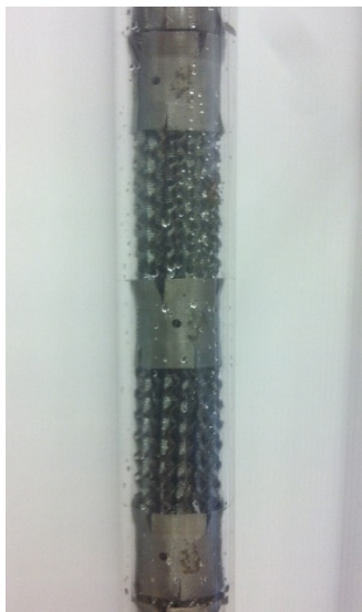
Figure 4.15: The stripping column with the structured packing FLEXIPAC 700Y
