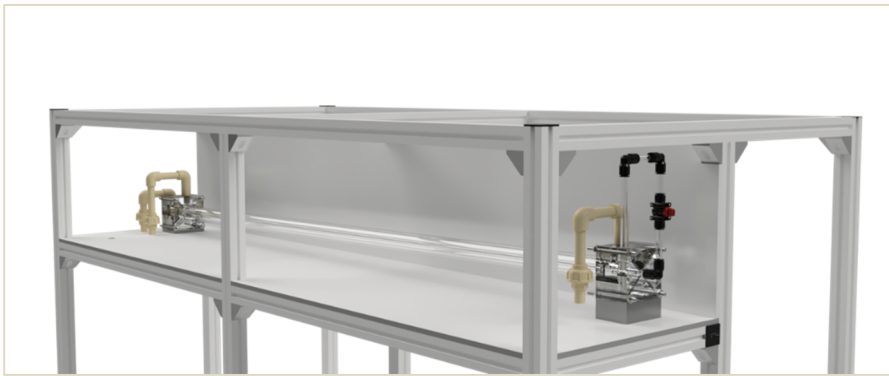
Figure 9.10: New MF-PFR reactor rendering made with Autodesk Fusion360®.
