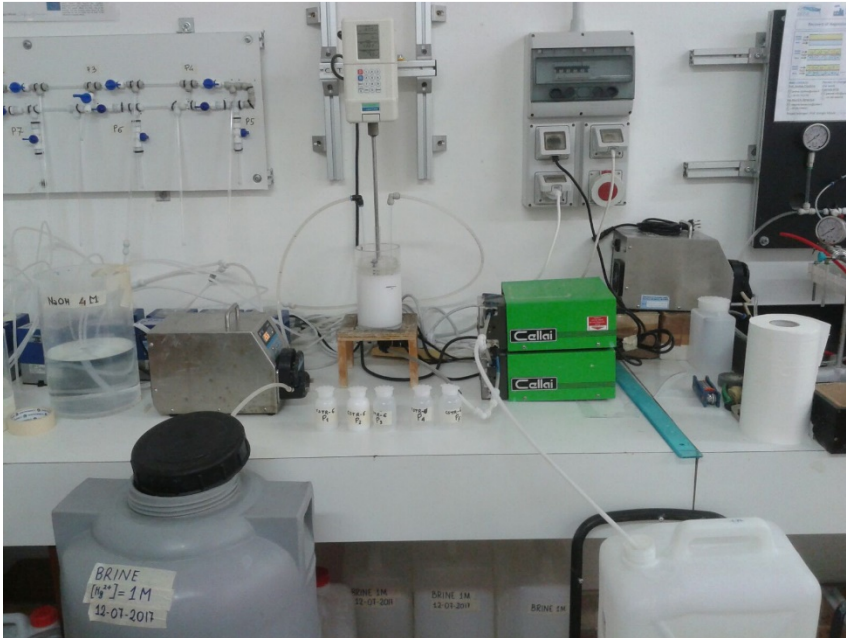
Figure 9.2: CSTR lab test-rig.
