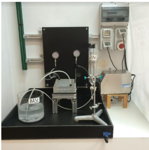
Figure 8.23: Experimental set-up with the third version of CriEM (v03).
