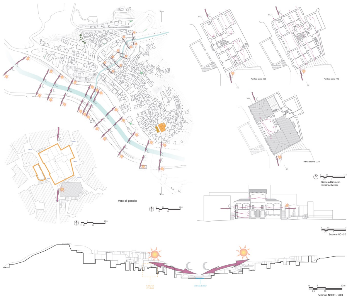
Figure 10. Air movements' multi-scale analysis: slope winds at district and building scale. Preparatory study for master diploma design of intervention on an historical building in Sinagra (M. Bonina, 2017).
