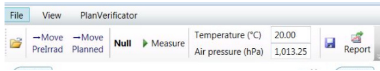
Figure 4.13: The tool bar at the top of the Plan Verificator contains all tools required to execute a verification. In evidence the temperature and pressure text fields.
