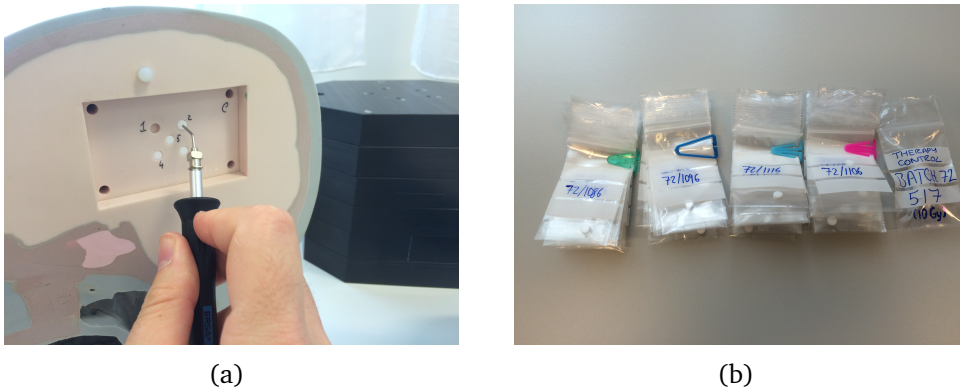
Figure 5.9: (a) Handling of the Alanine pellets with a dedicated vacuum tweezers. (b) Numbered bags containing individually irradiated Alanine pellets. In the picture also the control dosimeters encapsulated in a Delrin container are shown.
