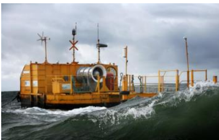
Backward Bent Duct Buoy (1:4th of full scale, tested in Galway Bay, Ireland, 2008.
