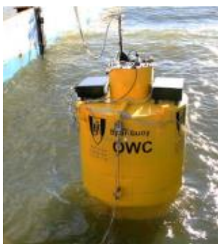
Model (1:10th-scale) of Spar-buoy tested in 2012 at NAREC, UK
