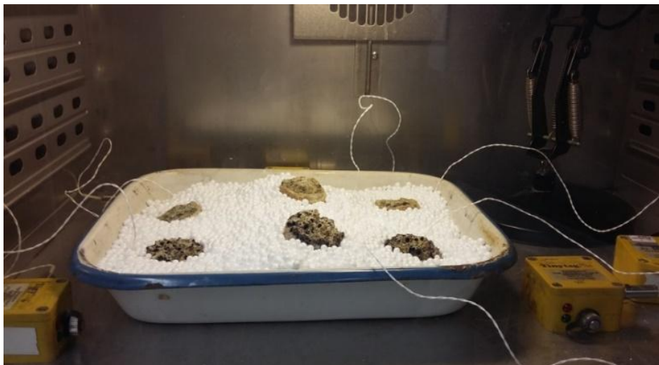
Figure 17, Core samples during a low tide simulation.
