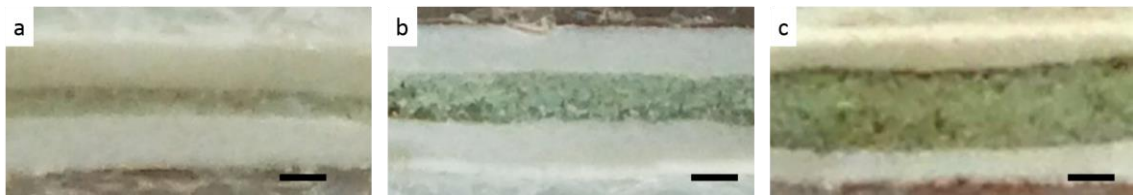
Figure 51 - Digital photo of sections of the multi-phasic laminates with the PLA core layer green colored. a) PCL laminate with PLA core 0.5 mm thick (LAM_0.5); b) PCL laminate with PLA core 1 mm thick (LAM_1); c) PCL laminate with PLA core 2 mm thick (LAM_2). Scale bar is 1 mm.
