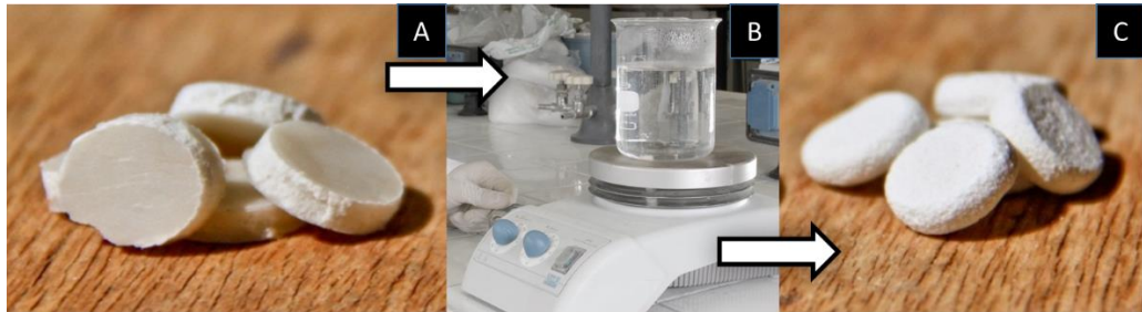
Figure 5 - A) Blend before leaching; B) Leaching step in demineralized water; C) 3D porous structures after leaching and drying in fume hood.
