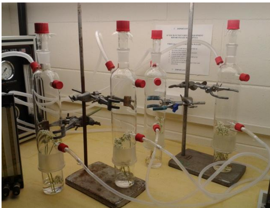
Fig. 5 Volatile collection system. Example of volatile organic compounds collection from buckwheat flowers.
